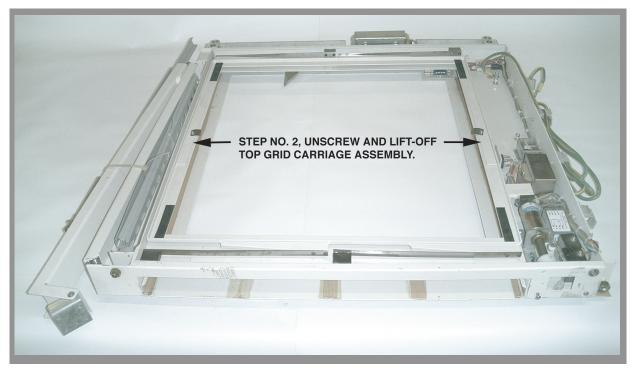
Step no. 2, unscrew four screws located at corners of grid carriage assembly and lift-off assembly. Do not discard assembly or screws.
