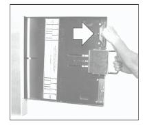
1. REMOVE SHELF FROM RETAINER BY ROTATING FLANGE FORWARD.
